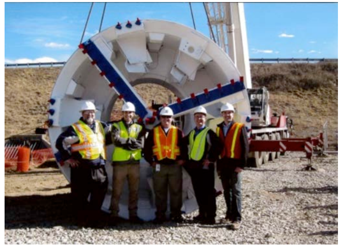
One hundred and eight inch tunnel-boring machine.
