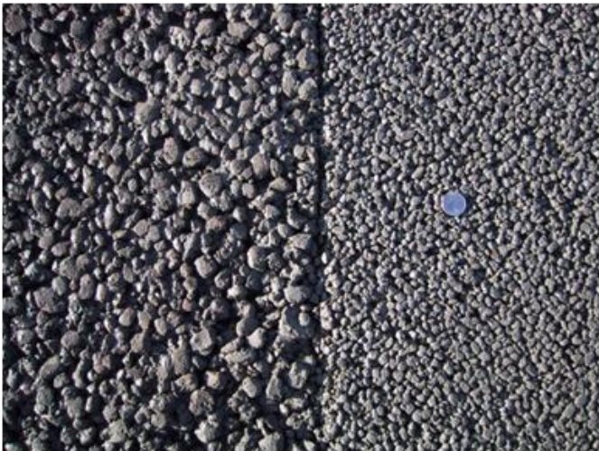
Photograph 1. The installation included two mixes utilizing different aggregates, AASHTO #67 (left) and AASHTO #8 (right).
