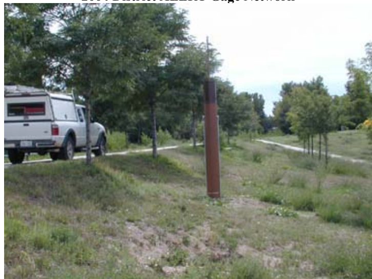
New ALERT rain/stage gage at Iliff Pond side channel detention basin on Goldsmith Gulch in Denver
